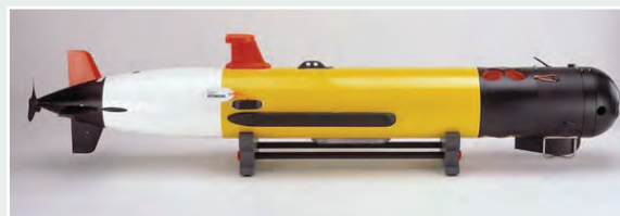
U.S. Navy AUVs, like the REMUS 100, are well suited to detect derelict fishing gear. NOAA and the U.S. Navy will demonstrate new uses of this technology and its value to marine scientists, fishermen and managers. Image: www.hydroid.com
